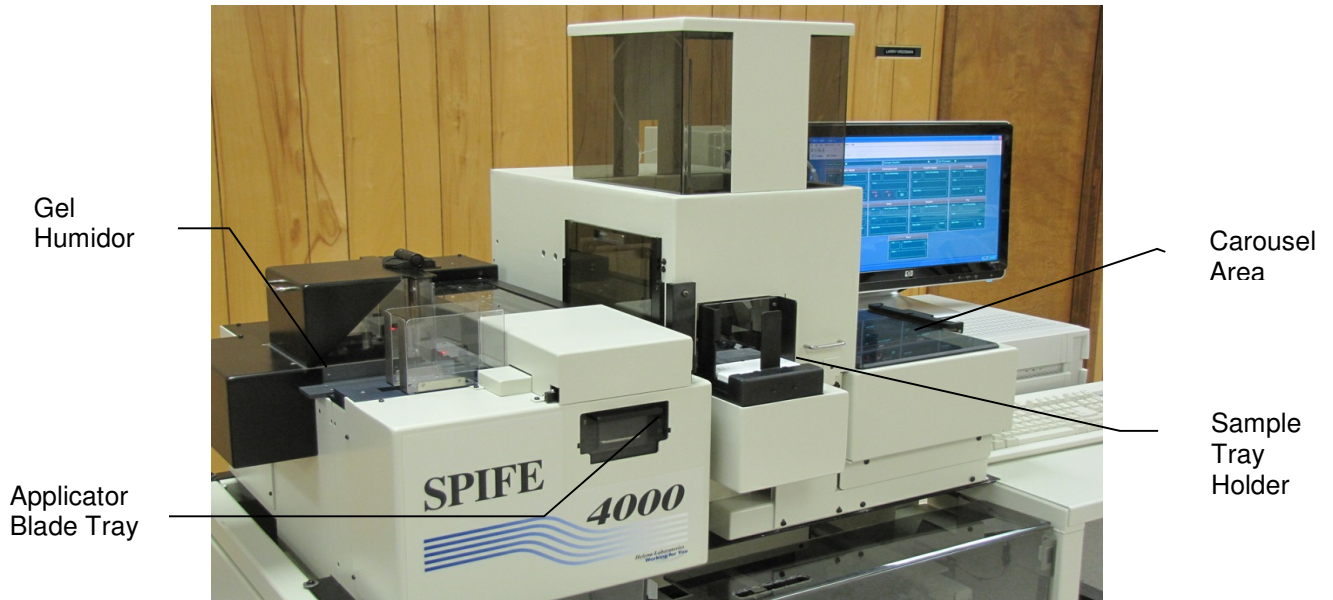
Figure 7-21 Sample Handling Area
